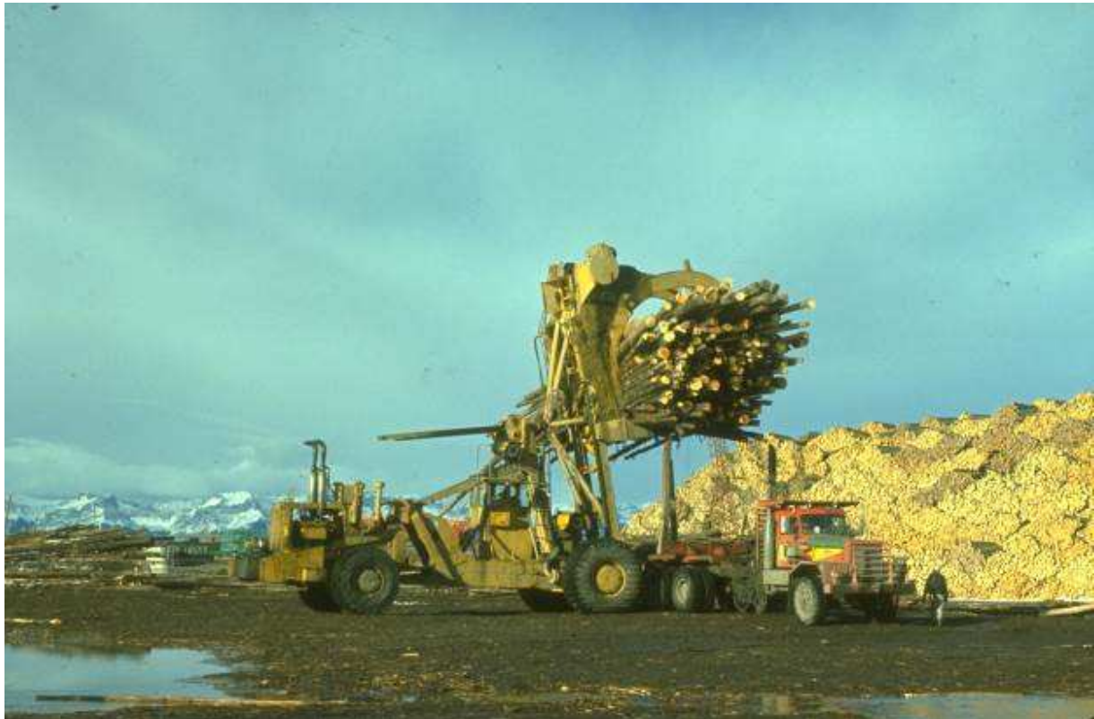
BEGINNING OF A NEW ERA, 1968: UNLOADING TREE LENGTH LOGGING TRUCK USING "CARRY-LIFT" THE LAST PILE OF 8-FOOT WOOD IS IN THE BACKGROUND
