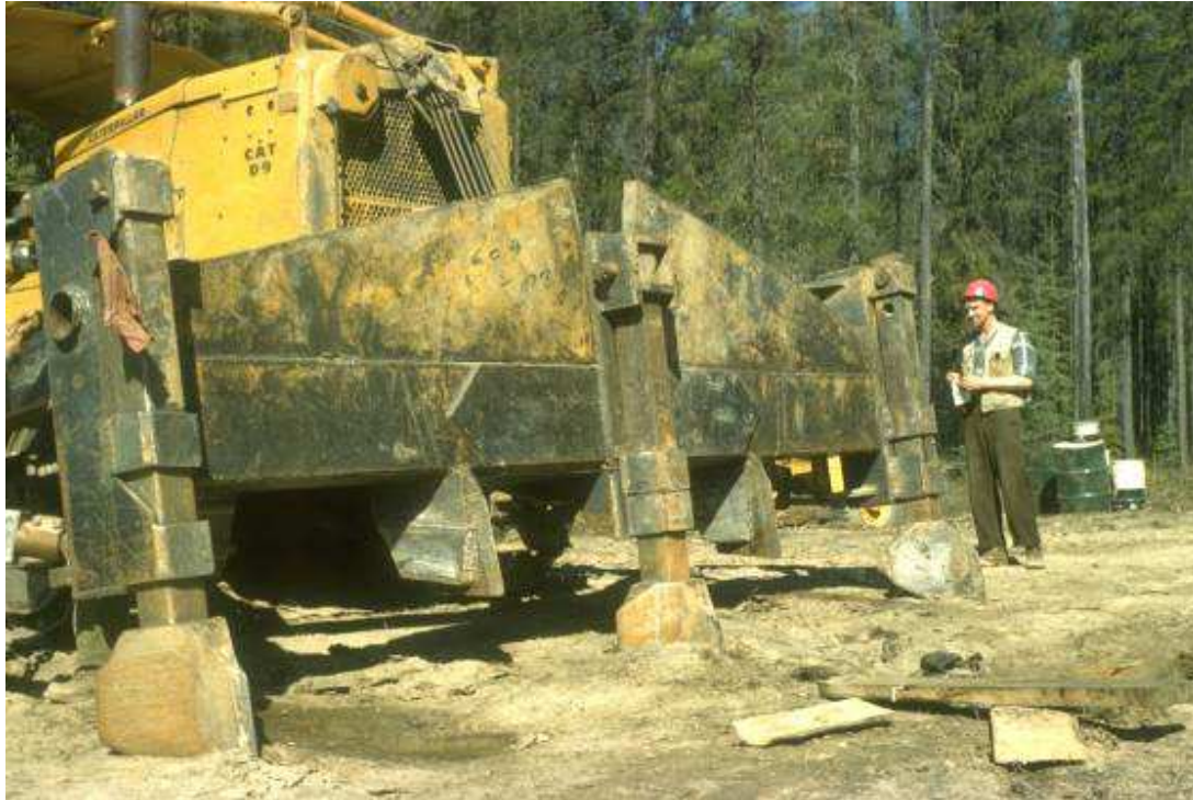
FORESTER OWEN BRADWELL EXAMINES SCARIFICATION PLOUGH MOUNTED ON A D-9 CAT, 1959 WELDWOOD PHOTO COLLECTION
