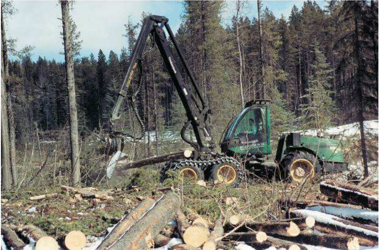
STUMPSIDE PROCESSING WITH SCANDINAVIAN-TYPE CUT-TO-LENGTH PROCESSOR
