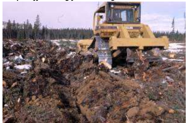
Site Prep for Planting with Craig-Simpson Ripper Plough
