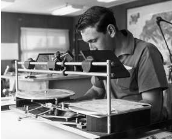
DRAFTSMAN ED STARKO USING A STEREO PLOTTER TO TRANSFER DATA FROM INTERPRETED PHOTOS TO A MAP BASE, CA 1960
