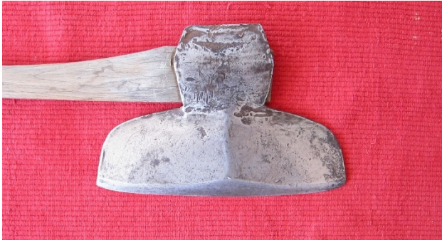
Two Views of a Broadaxe: The beveled side (left) is shaped like a normal axe, and used for chopping and roughing out the tie. The hewing Side (right) has no bevel and is used to chop out a perfectly flat side such as was needed for square timbers or railroad ties. Photo: Bob Udell
