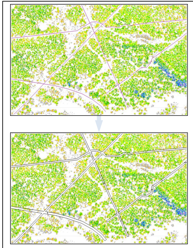
Figure 3. Example showing poly-lines being converted to polygons The Canopy Height model is based on a 1 meter grid with heights coloured into 3 meter height classes
