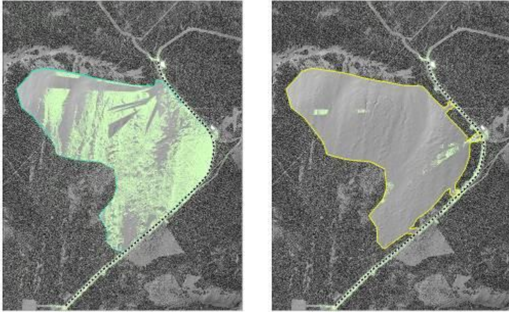
Figure 13: Sightlines (green) from roadside (dashed) with timber visual buffers (right) and without (left).
