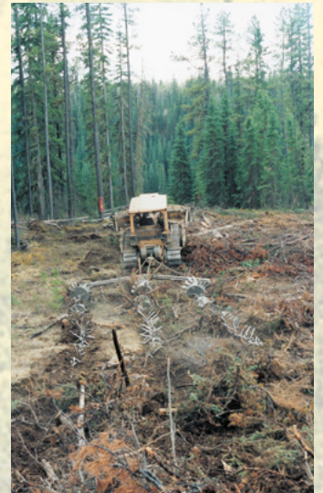
Adaptations of drag scarification techniques continue, such as this combination of shark-finned barrels and anchor chains.
