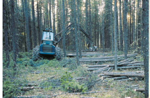
Feller-processors are used for commercial thinning operations.
