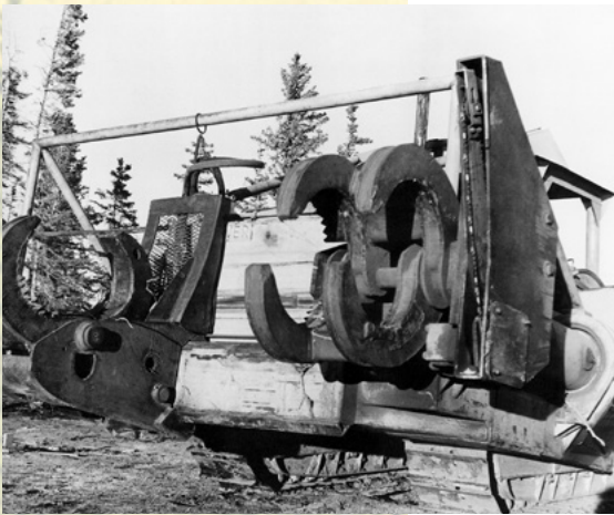
One of the earliest known prototypes of the modern-day feller-processor, the Pope Harvester is shown during field trials in 1957–58.
