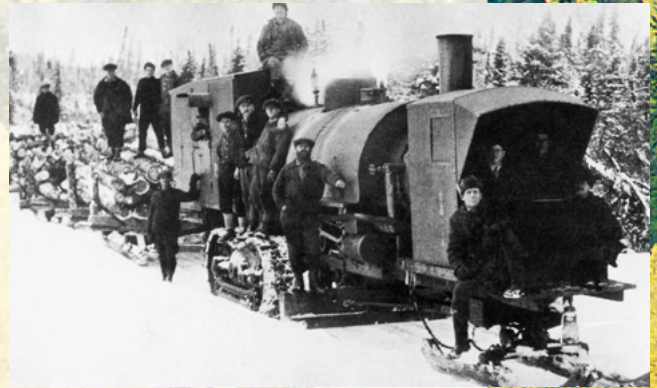
The Corser sawmillers crew used a steam sled for this winter log haul near Edson in the early 1940s. CORSER COLLECTION, UNIVERSITY OF ALBERTA ARCHIVES
