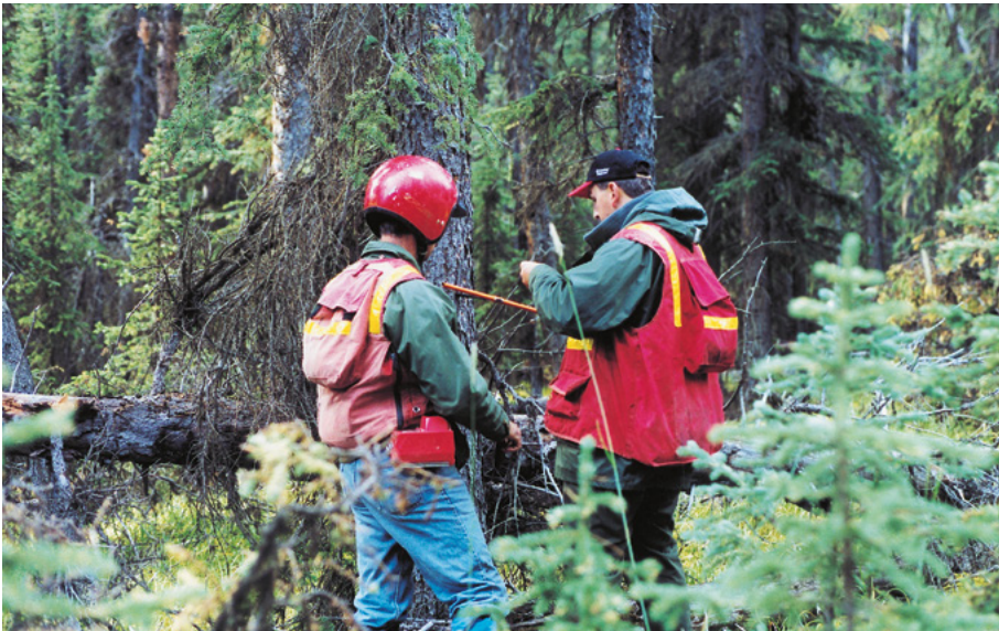
Company forester Ritchard Laboucane uses an increment borer to extract a small cylinder of wood from a tree, from which he derives the tree's age and growth rate by counting the growth rings.
