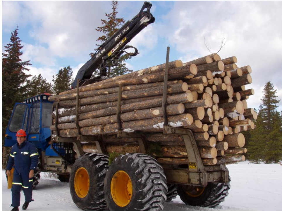
Figure 6-6: Low-impact wheeled forwarder used during Jasper project.
