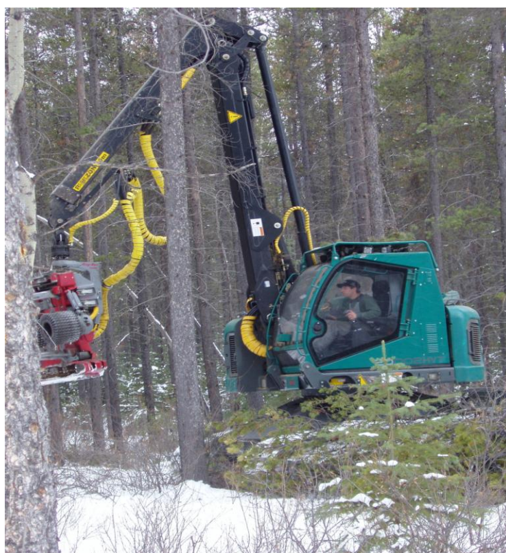
Figure 6-5: Small, maneuverable wood processor used for selective thinning in Jasper project.
