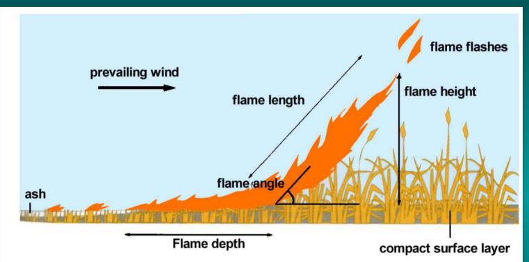
Simple Formula for Field Use (For surface fires & intermittent crown fires)  $I = 300 \ge (L)^2$ L = Flame Length (metres)
