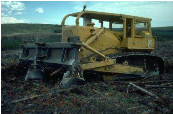
Crossley Scarifiers on D9 Tractor, 1976 - Final Design HINTON WOOD PRODUCTS COLLECTION
