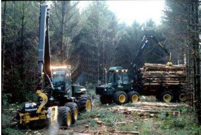
Timberjack harvester and shortwood forwarder in Southern Pine plantation. The abundant lighting enables both day and night operations. With the high cost of equipment, double-shifting is often a necessity.
