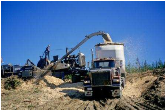
Bush Chipping Operation, McLeod Compartment 7, 1993. Full trees were chipped, the branches, bark and needles separated from the wood chips which were then blown into vans for transport to the mill. The chipped-up branches, bark and needles were loaded into a machine similar to a manure spreader, but much larger, and spread across the cutover area.
