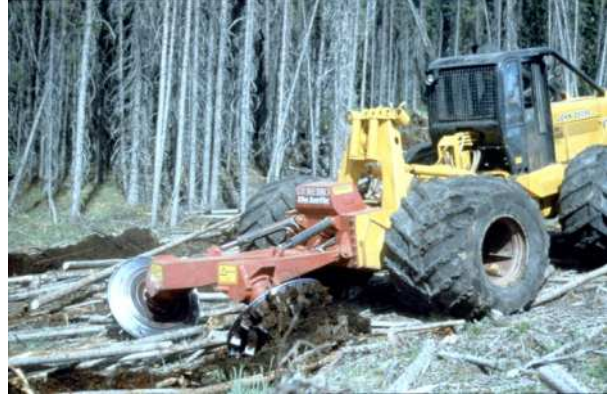
Modern site preparation equipment – Barrel and chain scarifier (left) and Disc trencher (right). Better utilization, including dead wood, leaves less debris and deadwood on the cutover areas, and lighter equipment such as that shown can be used effectively to prepare sites for natural seeding or planting
