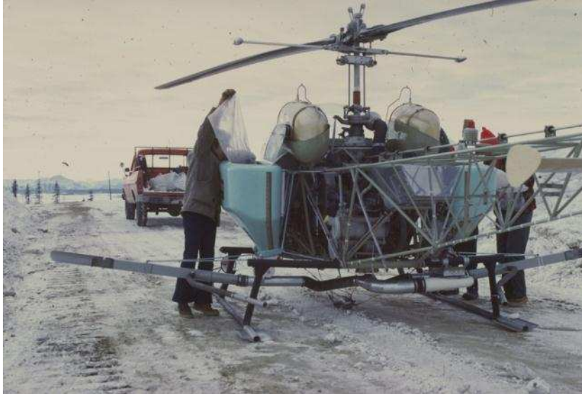
Loading seed into Brome Seeder on Bell G3 Helicopter, 1973
