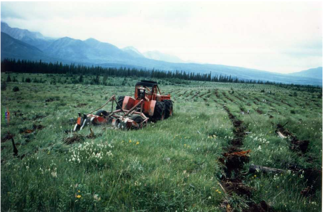
Bracke Scarifier working at Camp 1, 1970s
