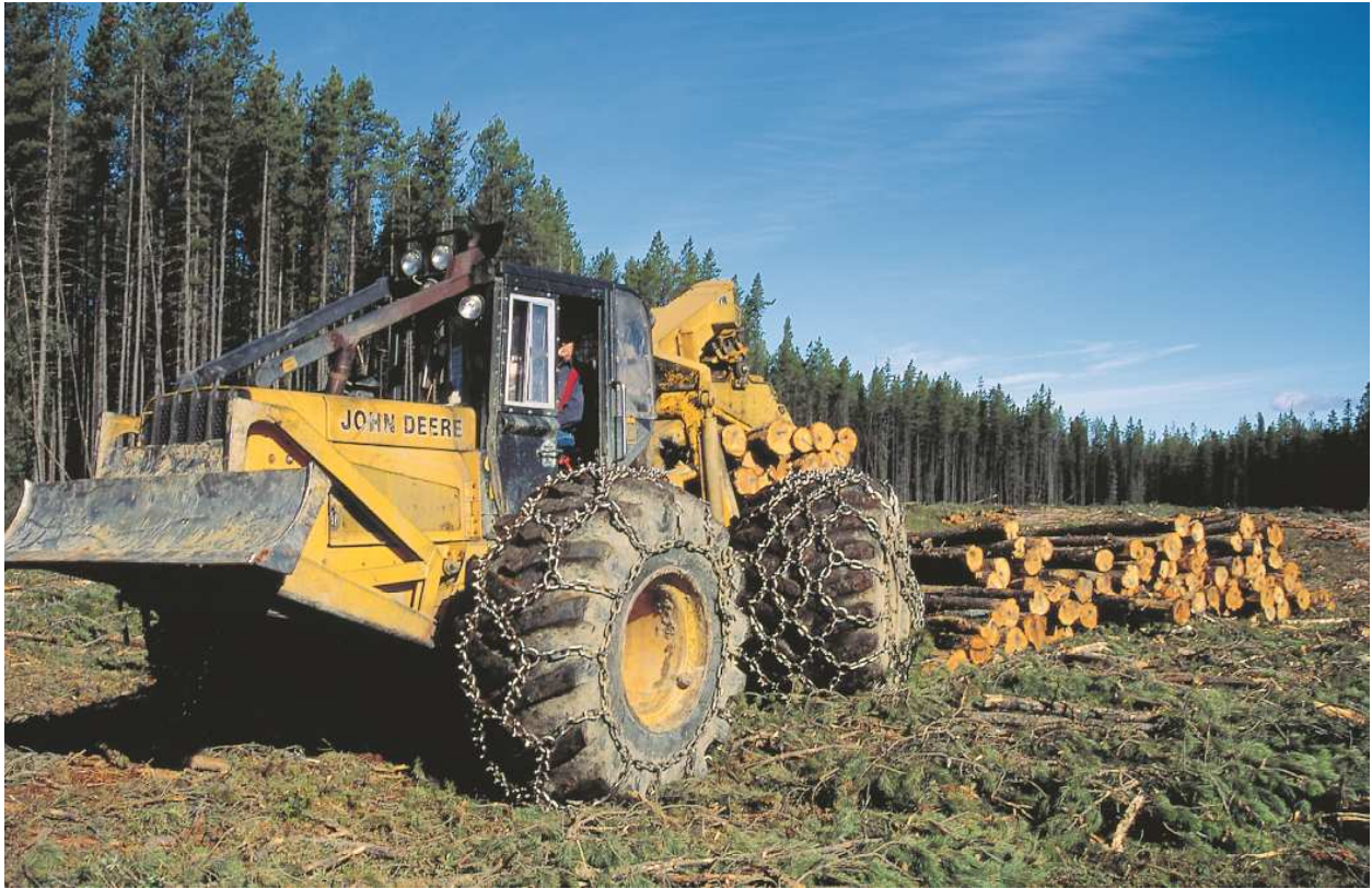
Grapple Skidder with high-flotation tires, 1990s. Note the mat of branches on the cutover, which also assists flotation. HINTON WOOD PRODUCTS COLLECTION
