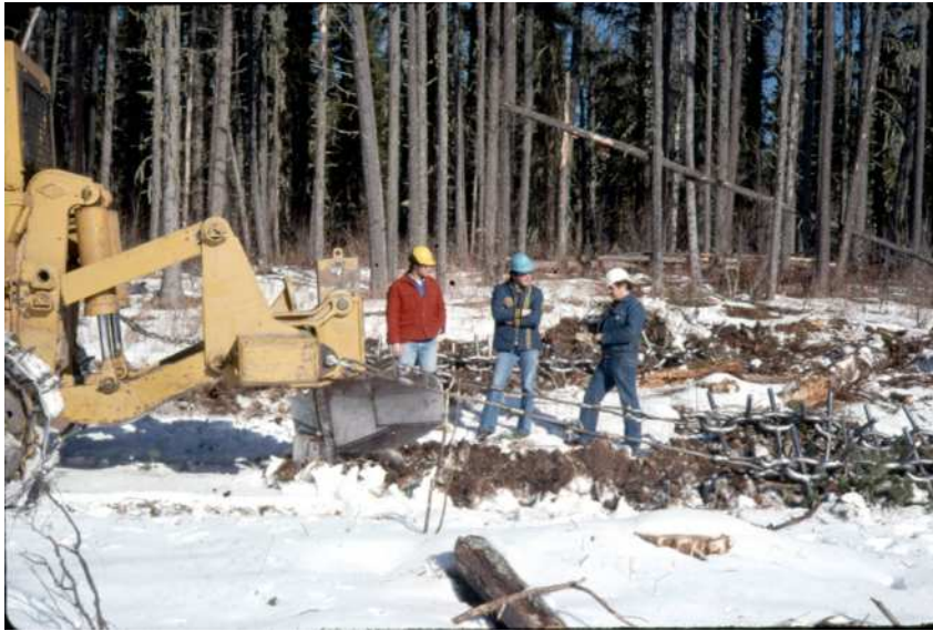
C-S plough with chain drags for natural regeneration, 1980s HINTON WOOD PRODUCTS COLLECTION
