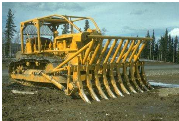
Early scarification equipment: Flecco Rake (l), 1956 and scarification plough on D9 tractor (r) 1959 with Forester Owen Bradwell
