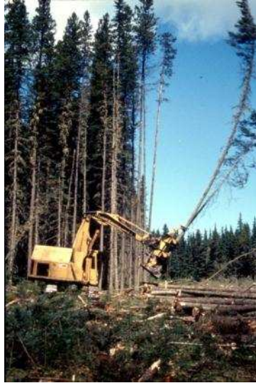
Feller Buncher and Grapple Skidder, late 1980s HINTON WOOD PRODUCTS COLLECTION
