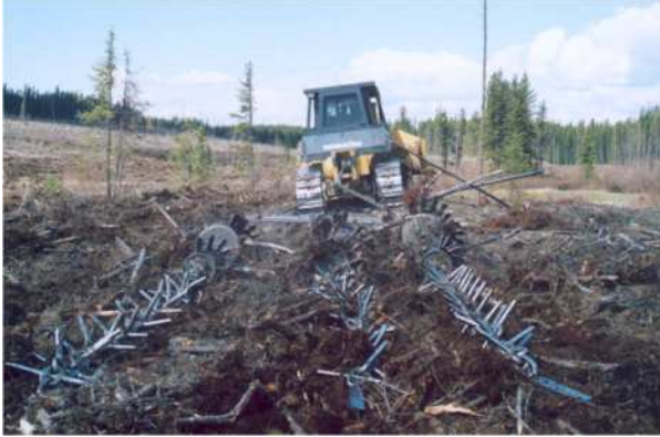
Modern site preparation equipment – Barrel and chain scarifier (left) and Disc trencher (right). Better utilization, including dead wood, leaves less debris and deadwood on the cutover areas, and lighter equipment such as that shown can be used effectively to prepare sites for natural seeding or planting
