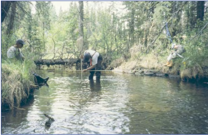
Measuring bankfull depth from measuring tape elevation.
