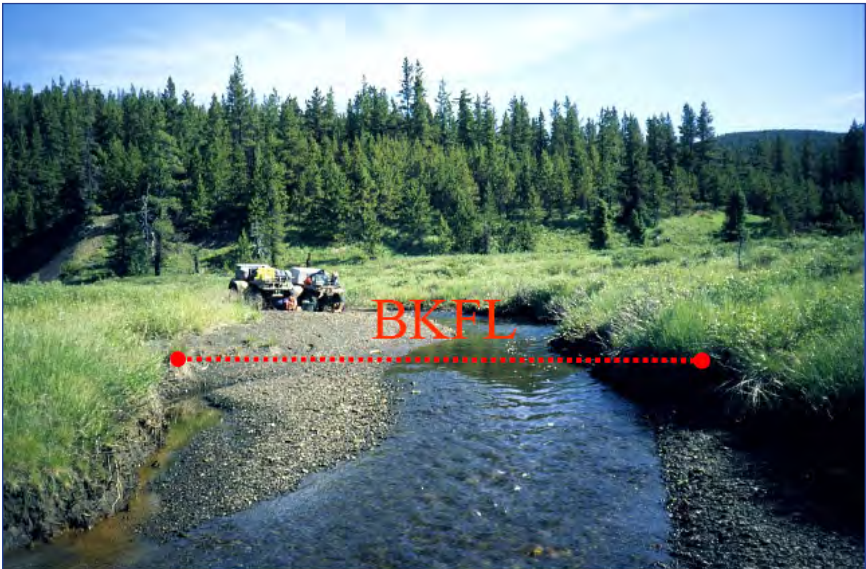
A suitable site for measuring bankfull width in a straight riffle section away from bends and pools.
