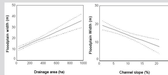
Figure 9. Predicted floodplain width and 95% confidence intervals for range of drainage area and reach slope values.
