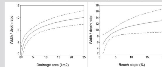
Figure 14. Predicted width/depth ratio and 95% confidence intervals. R<sup>2</sup> = 0.692.
