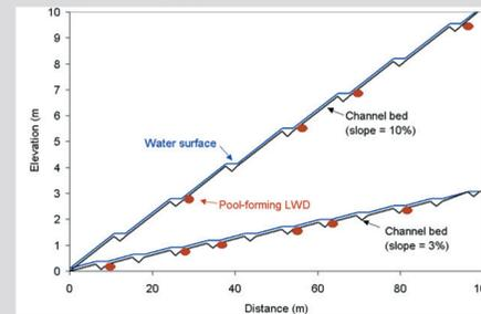
Figure 13. Longitudinal profiles of two headwater streams (3% slope and 10% slope) with pool extent, pool frequency and LWD function.
