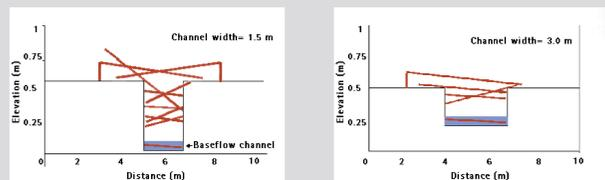
Figure 2. Channel cross sections for a 1.5 m wide stream and a 3.0 m wide stream showing different ratios of in-channel / baseflow-channel LWD.
