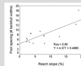
Figure 11. Model for predicting pool spacing (channel widths/pool) from reach slope (%).
