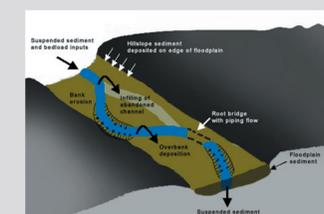
Figure 21. A sediment budget for a stream within a glaciated headwater valley (adapted from Reid and Dunne, 2003).
