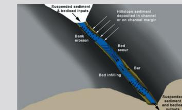
Figure 20. A sediment budget for a stream within a V-shaped valley (adapted from Reid and Dunne, 2003).
