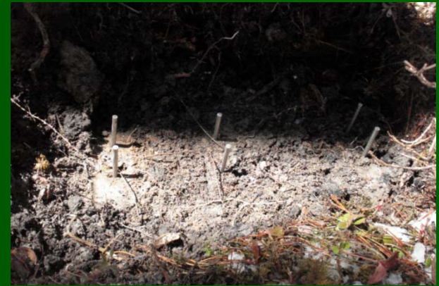
Spot measurements soil moisture (TDR)
