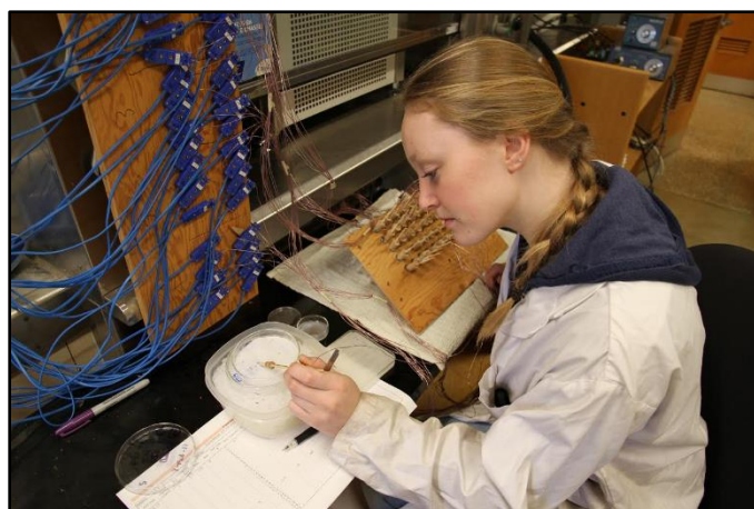
Assessing the cold tolerance of MPB by measuring the super-cooling point of individual insects.
