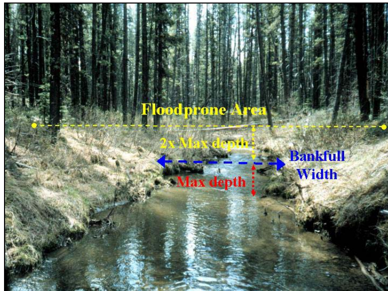
Figure 1. Determining floodplain width on a foothills stream with a lodgepole pine dominated riparian area.
