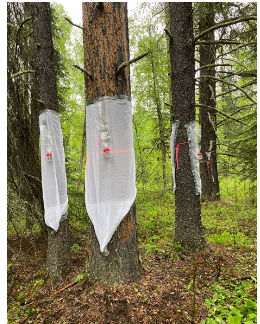
Flight intercept, emergence, and landing traps set up on trees.
