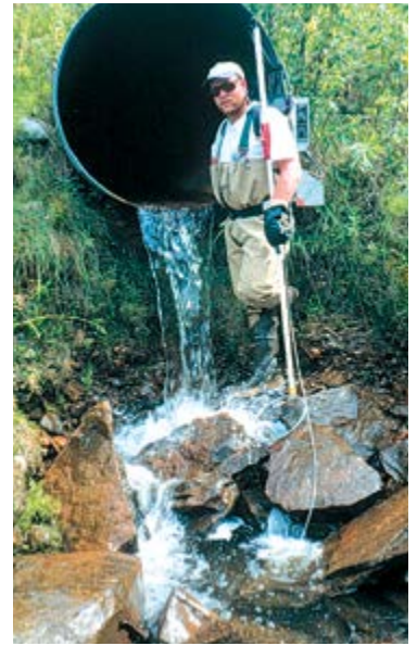
FMF fisheries biologist Cam Davis inspects a hanging culvert, 1998. Hanging culverts such as this one are major impediments to fish passage.
